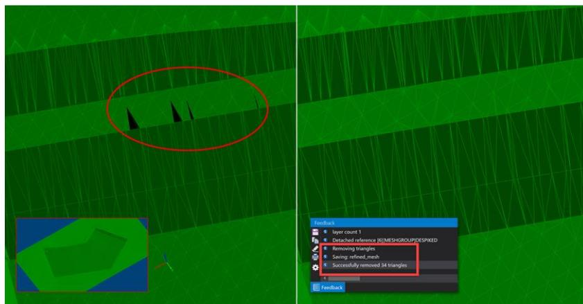
*Before and After Comparison of a Successful Despiking Function*
